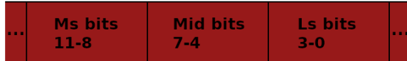
Figure 2. Address storing convention for virtual address registers with most (resp. least) significant nibble first (res. last).
